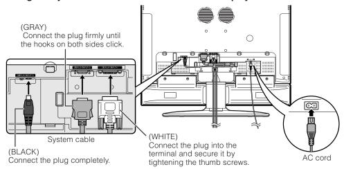
3 Connecting the system cable and the AC cord to the AVC System
